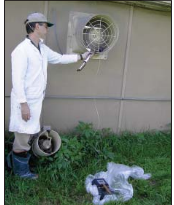
Figure 1. Using colorimetric tube to measure ammonia from barn fan
