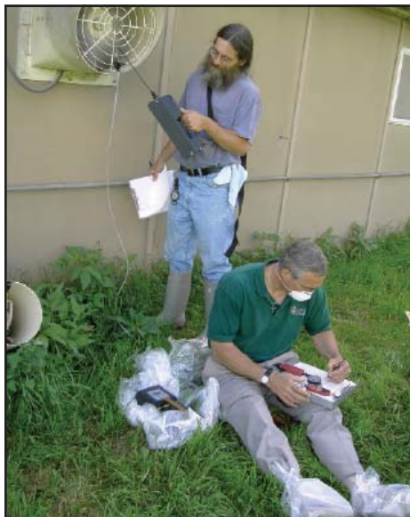
Figure 2. Using Jerome Meter to measure hydrogen sulfide
