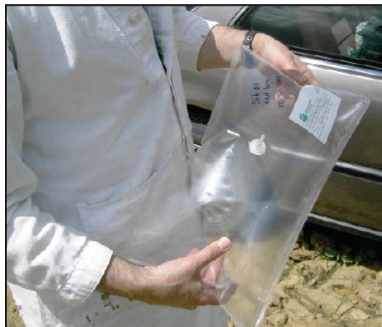
Figure 3. Bag of air collected and delivered for lab analysis by dynamic olfactometry
