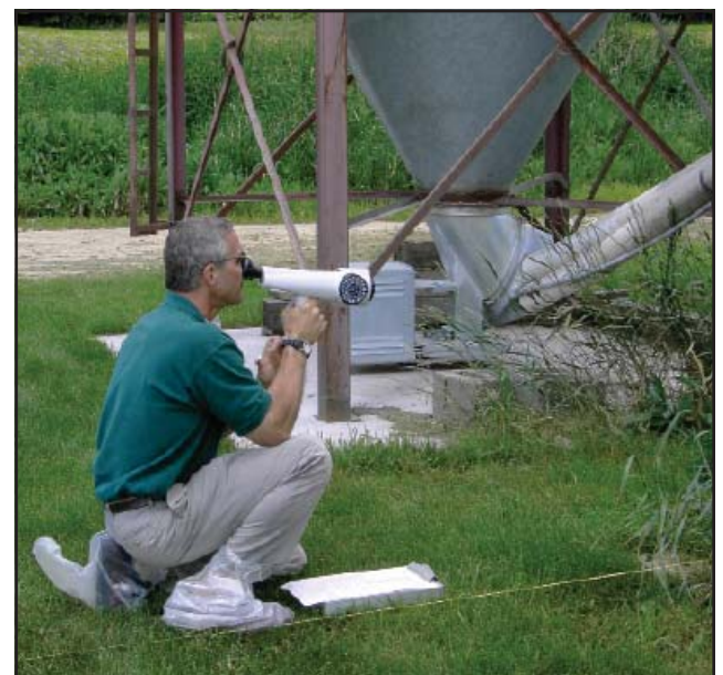
Figure 4. Using Nasal Ranger Olfactometer to measure odors
