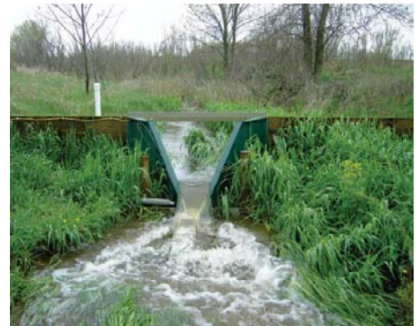
Flume at a Discovery Farms monitoring station.
